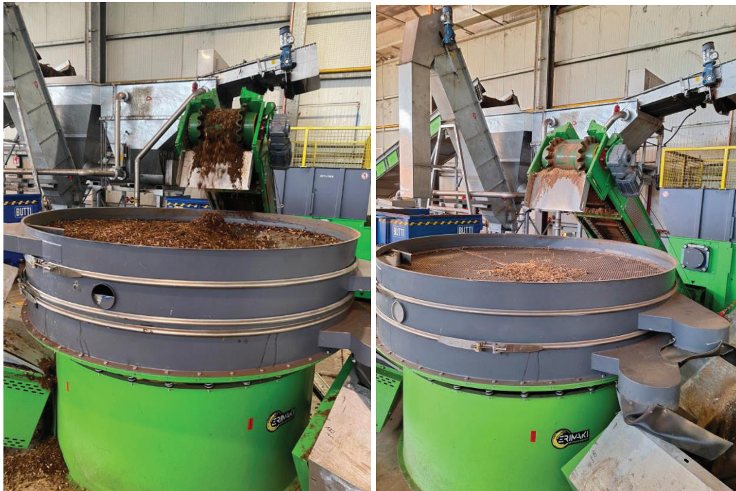
Fig. 6 – Fine screening operating after the shredder belt
