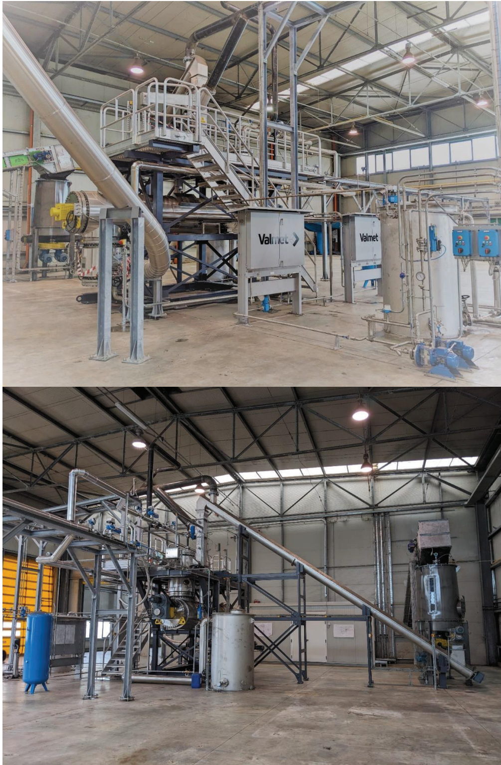
Fig. 7 – complete steam explosion system on site
